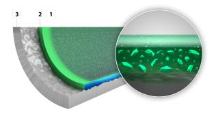
XERADUR 3 is an one or two-layer sol-gel system. The product convinces with a very good long-term non-stick effect as well as best abrasion resistance. XERADUR 3 shows absolutely no cracking or staining. The glossy surface gives the coating a noble touch.
