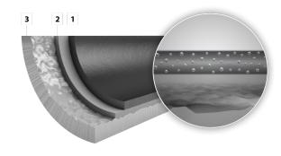
CORFLON Ultra is a two-layer system that is particularly suitable for small electric appliances used to process bread dough or for electric cookware.
