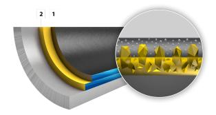
ILAFLON Resist R Plus FF is a strongly ceramic reinforced system with excellent performance in abrasion resistance, durability of non-stick effect and cleanagility. For top level baking and roasting applications
