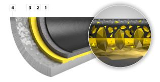
Durit Protect Pro is a three-layer non-stick system coating with ceramic reinforcement for highest - ideally suited for use with top level cookware in particular. Due to an excellent combination of scratch- and abrasion resistance with best nonstick, it is the system of choice.
